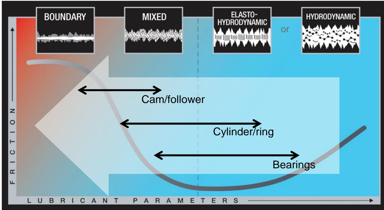
Hardware changes, down-speeding and using lower viscosity oils are increasing the time operating in the boundary regime
