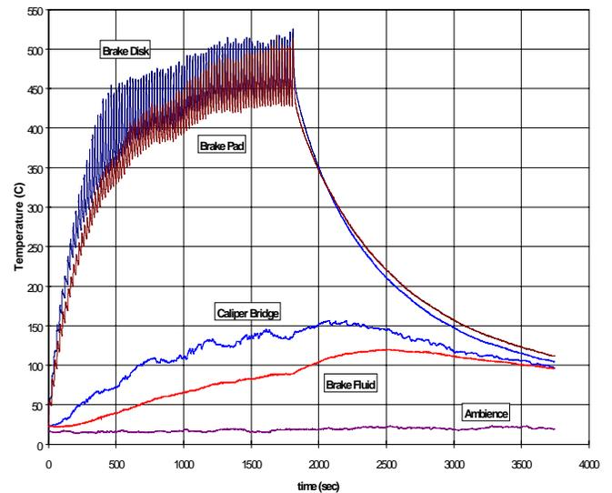
Figure 8. Measured temperatures during a repeated braking and heat soaking
