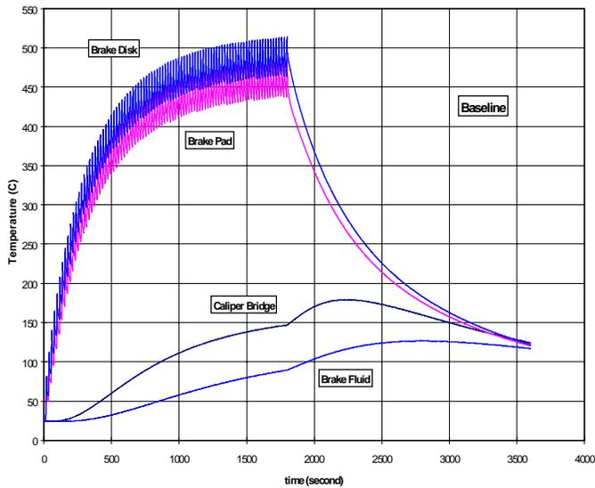
Figure 9. Calculated temperatures during a repeated braking and heat soaking
