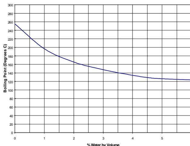
Figure 1. Boiling point vs. water content of DOT 3 brake fluid
