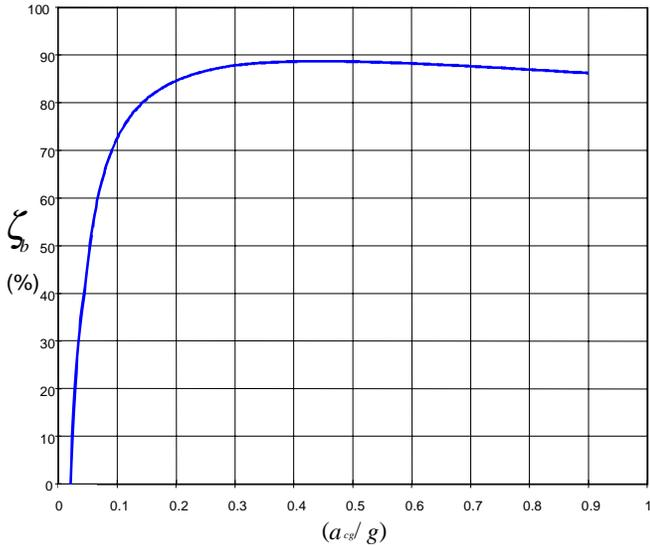
Figure 3. The fraction of power dissipated by the friction brakes
