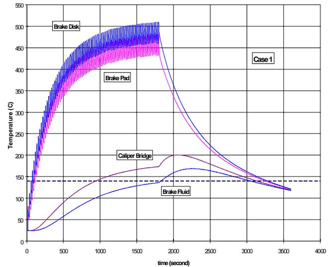
Figure 10. Calculated temperatures for the brake system with aluminum caliper and semi-metallic lining materials (Dashed line indicates wet boiling point)
