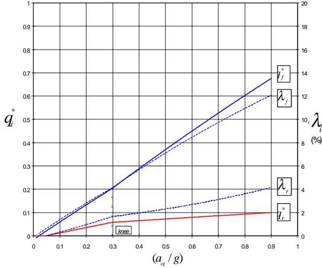
Figure 2. Brake power generation and tire slip
