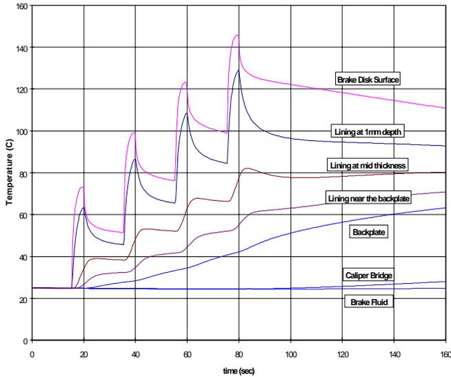
Figure 6. A transient simulation result for various brake components
