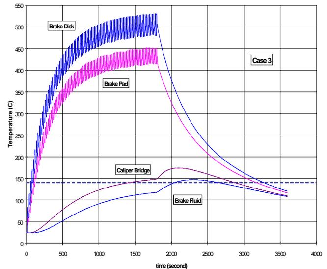
Figure 12. Calculated temperatures for the brake system with aluminum caliper and two thirds worn NAO lining materials (Dashed line indicates wet boiling point)
