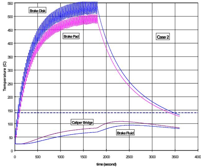
Figure 11. Calculated temperatures for the brake system with aluminum caliper and NAO lining materials (Dashed line indicates wet boiling point)
