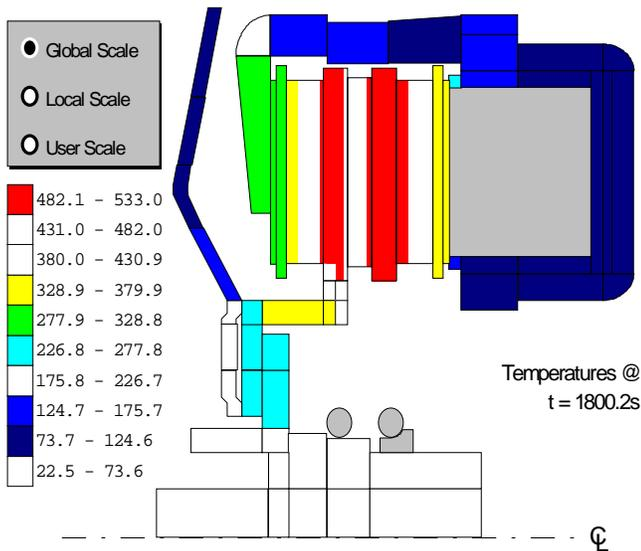
Figure 7. Graphical representation of temperature distribution in the disk brake system
