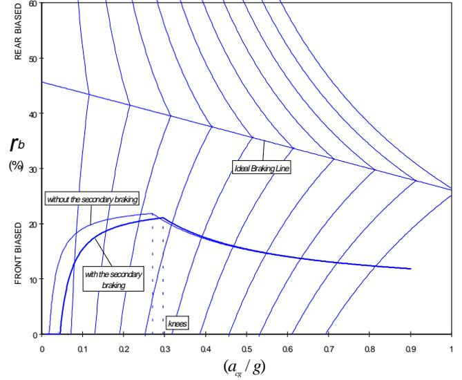
Figure 4. The effect of secondary braking on the brake balance
