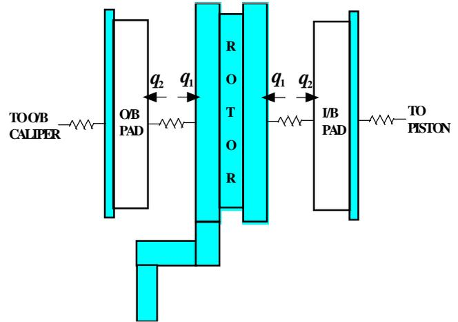
Figure 5. Heat balance at the friction interfaces
