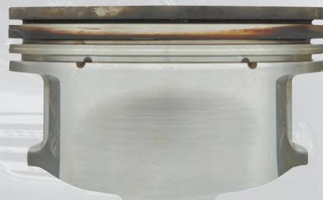
Piston After Double-Length Sequence IIIG Engine Test
