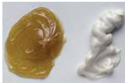
Figure 3 | One of the applications that shows promise for a new boron nanoparticle-based lubricant additive is in lithium complex greases. In one application, the additive was able to replace the entire antiwear/extreme pressure additive package in the grease leading to an increase in performance. [Courtesy of DRD Additives LLC]
