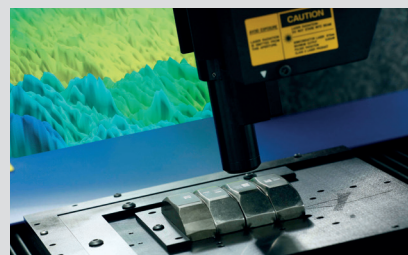
FIGURE 11: The optical profilometer uses a laser as a non-destructive way to measure wear. It is enabling Shell scientists to evaluate product wear performance more precisely than conventional methods.
