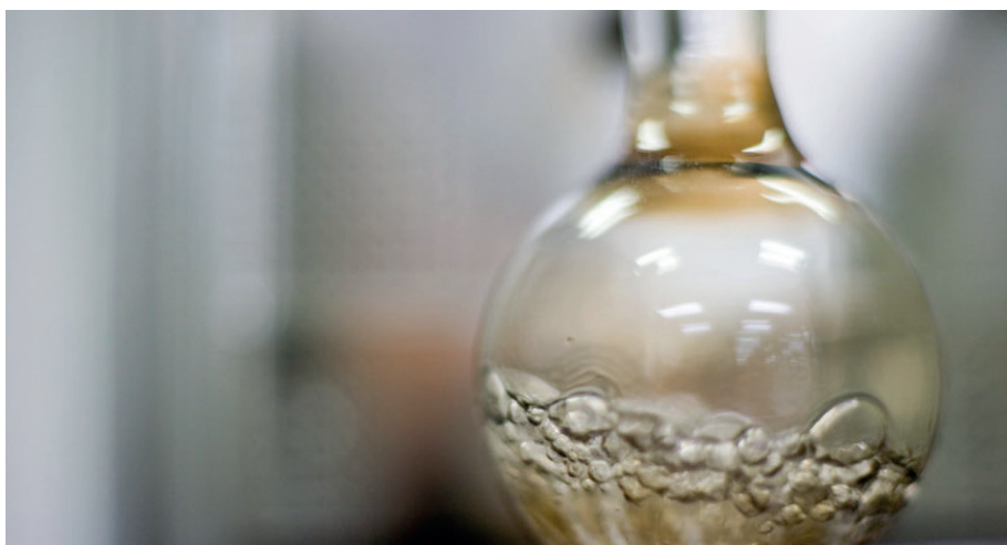
FIGURE 2: The formation of air bubbles in an oil formulation.
